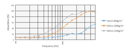
$SP\ Report\ P805432\ (\ 2008-11-06\ )\ Determination\ of\ sound\ absorption\ coefficient\ in\ impedance\ tubes\ according\ to\ ISO\ 10534-2$
